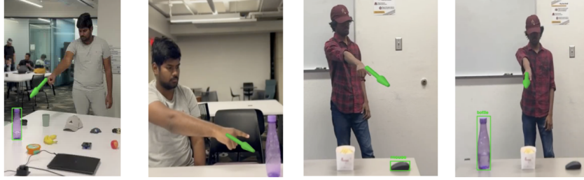
Figure 2: Model performance upon Pointing gesture arrow and object detection (a) True Positive (b) False Negative (c) False Positive (d) True Negative respectively
